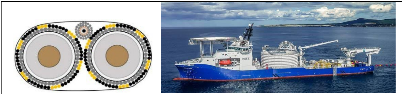
Figure 1-1 Illustration of the marine cable system (left). Cable-laying vessel NKT Victoria (right).
